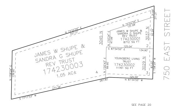
10' UTILITY & DRAINAGE EASEMENTS EACH SIDE OF PROPERTY LINES AS INDICATED BY DASHED LINES EXCEPT AS OTHERWISE SHOWN.
